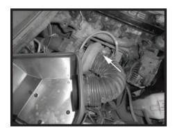
Step 10 Fully tighten the clamp on the turbo side of the intake tube.
