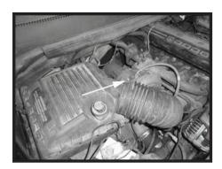
Step 2 Loosen the clamp on the factory tube to factory air box lid.
